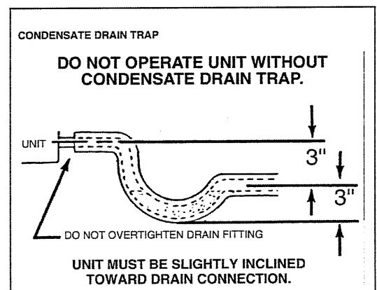
p) Install a "P" style drain trap on the condensation drain line as close as possible to the AHU.
